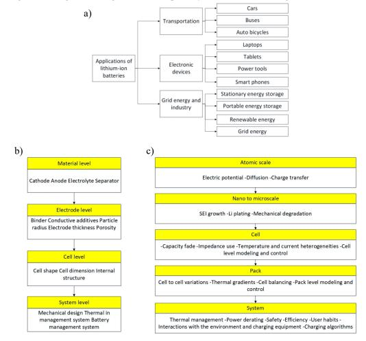
Fig. 1. Applications of lithium-ion batteries (a); lithium-ion battery design on different levels [9] (b); principal factors influencing lithium-ion battery rapid charging [10] (c)
