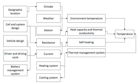
Fig. 2. Factors affecting the temperature of lithium-ion batteries [9]
