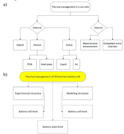
Fig. 3. Classification of different thermal management approaches [17] (a); organization of thermal management systems (b)
